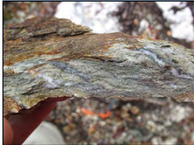
Figure 26: Golden Culvert sheared phyllite Sheared, silicified phyllite adjacent to Golden Culvert main showing; quartz veinlets crosscutting main foliation; note fine, acicular arsenopyrite needles.
