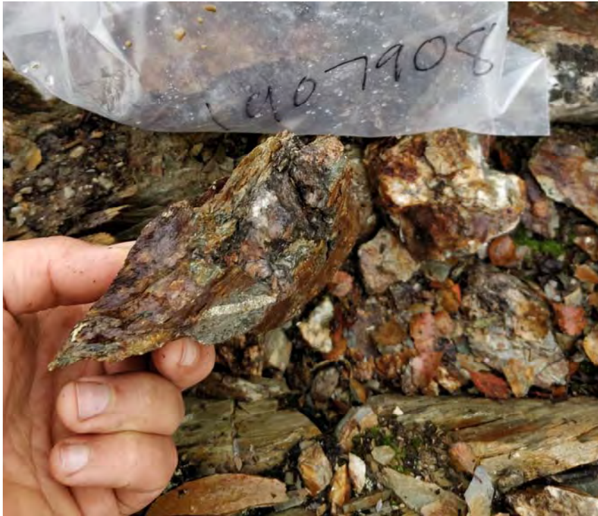
Figure 29: Sample 1907908 Golden Culvert main showing; arsenopyrite >2% in siliceous grey phyllite; assay of 2.5gpt Au and >10,000 ppm As.
