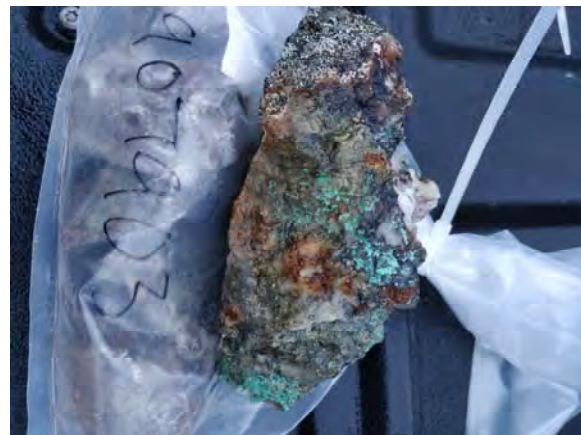
Figure 34: Sample 1907903 Green Dragon showing; quartz vein with disseminated chalcopyrite and malachite stain; assay of 6,575ppm Cu, 13,805ppb Ag.
